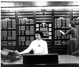
The Harvard Mark II Machine, an early computer boasting magnetic drum storage.
